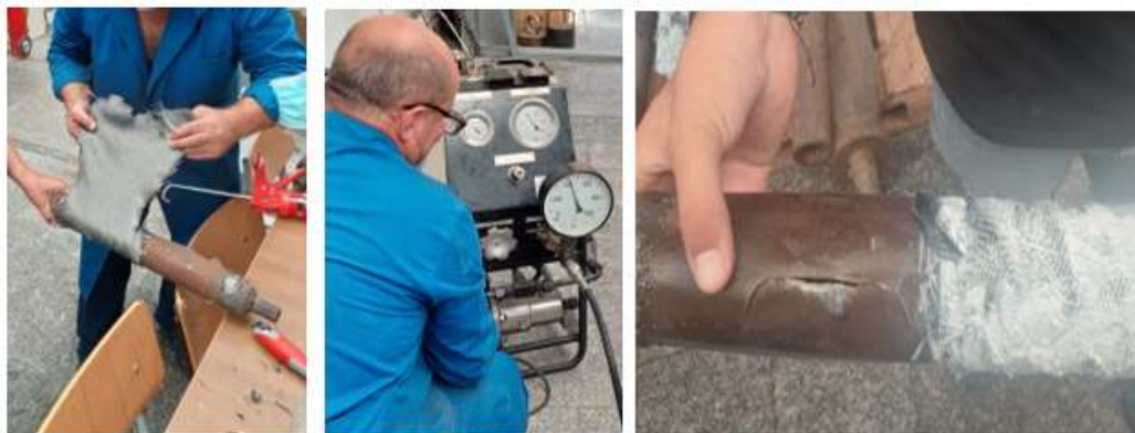
Figure 1. Burst pressure test of steel pipe repaired with composite epoxy-filled repair sleeves
