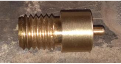
Figure 16 Brass Grade 360 Specimen
