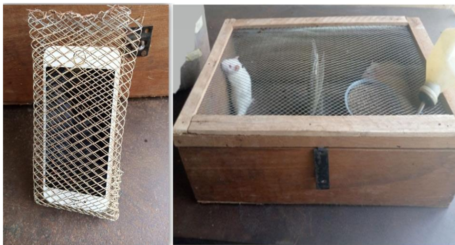
Figure 1: A phone wrapped with aluminum wire mesh and the cage (The exposure field)
