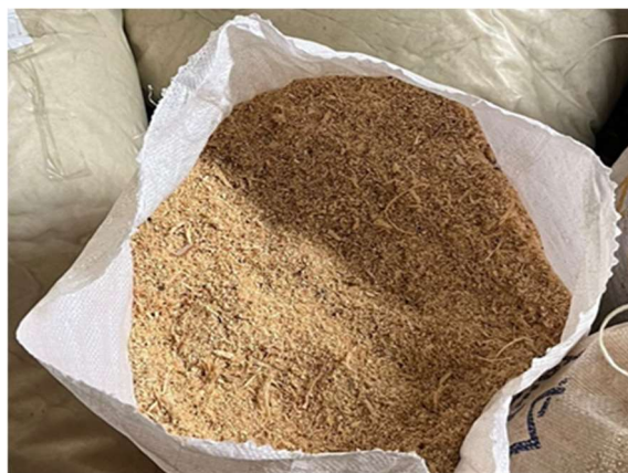
Figure 2. Ground apple tree pruning biomass prepared as feedstock for pellet production.
