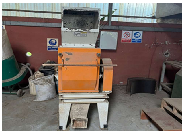
Figure 1. Hammer mill used for size reduction of apple tree pruning residues prior to pelletization.
