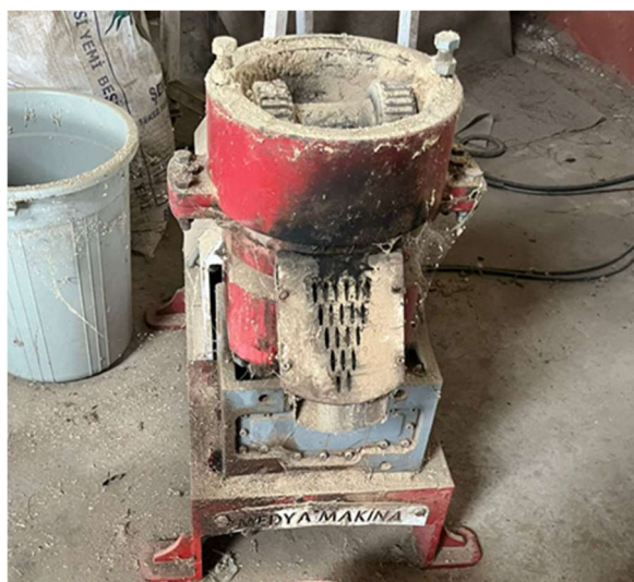
Figure 3. Laboratory-scale flat die pellet mill used for pellet production.
